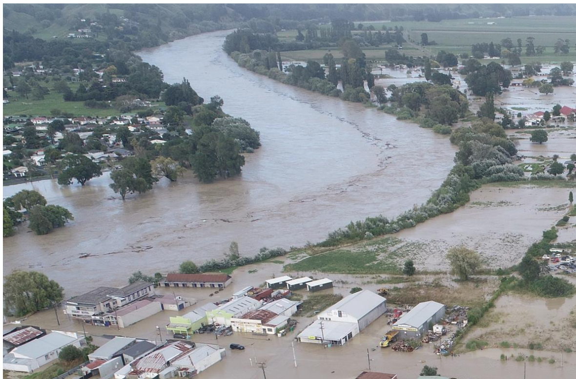
Figure 1 – LWD forming a line along the Wairoa River – this line typically follows the deepest part of the channel.
