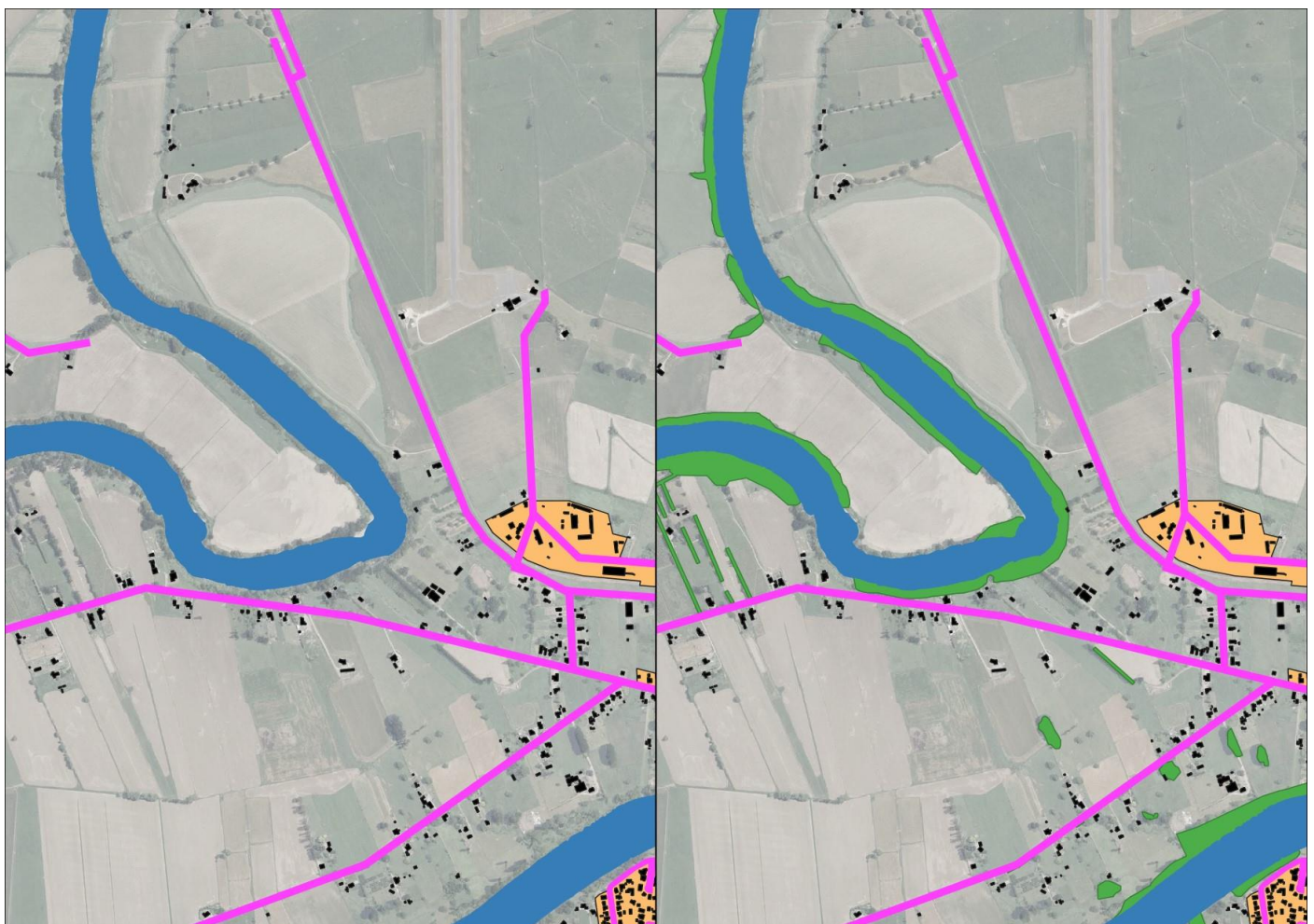
Figure 4. Roughness zones comparison - before incorporation of trees/scrub (left). After incorporation of dense trees/scrub (right).
